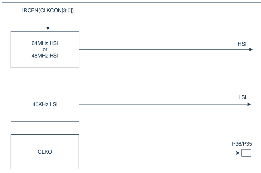
Figure 3-1: Block diagram of the clock structure
